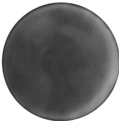
PLATE 1 Photographs of the thin film of \text{Pt}(\text{dpg})_2 under shear deformation at 0.4 GPa. The color of the thin film changes remarkably from green to yellow at the outer part, but the color at the center is green. The yellow region is remarkably observed at around about 75% of the radius ( 0.75r ). (See COLOR PLATE IV)
